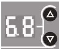
Press the two direction buttons **9** and **10** simultaneously. Then the automatic shut-off time can be set. A range of 0 - 60 min. is adjustable shown on the digital display **8** (disregard the decimal point, e.g. 0.2 means 2 min. shut-off time). Switching off automatically is signaled by a tone (3x) when AUDIO is switched on.
